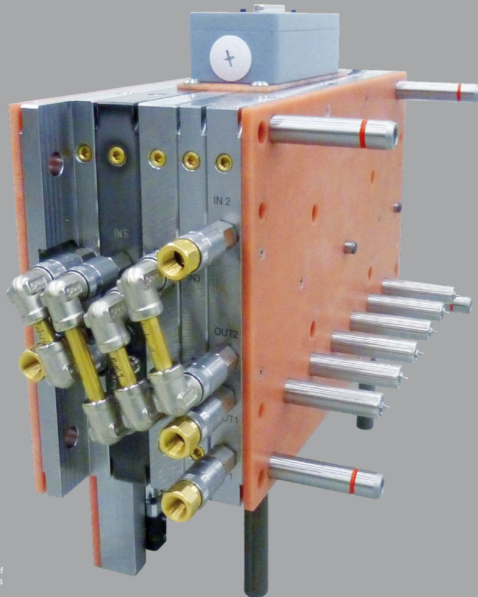
Customised 6 cavities cold runner for HCR processing
