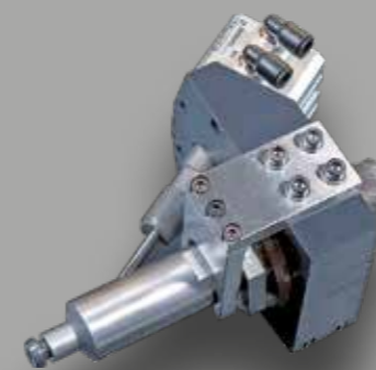
DIVING NOZZLE decouples the cold runner and the cylinder during metering by means of a valve gate.
