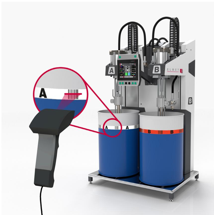
ELMET has now further enhanced operating safety in silicone injection molding. A barcode system developed jointly with the WACKER chemical group for the reliable differentiation between components A and B, plus a corresponding reading device on the TOP 5000 P dosing system reliably prevent any chance of confusion when changing drums – eliminating the danger of immense follow-up costs. © ELMET
