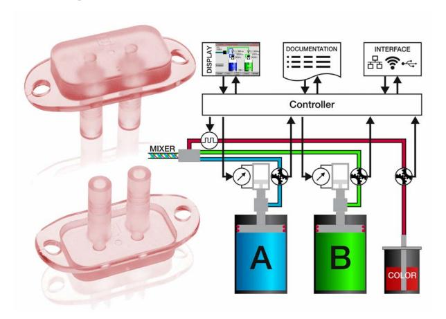
Combining a high-resolution flow meter with sensitive control and comprehensive documentation of additive and colorant metering, ELMET meets the stringent demands placed by the health-care industry on liquid silicone rubber injection molding.
