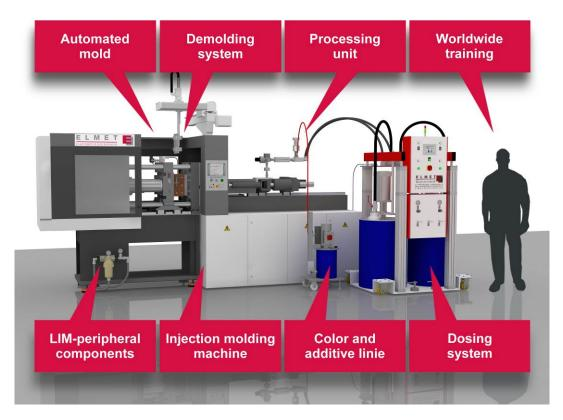
As a specialist for the entire field of liquid silicone rubber (LSR) injection molding, ELMET supplies custom-designed, fully equipped systems on a turnkey basis and thus assumes responsibility for the smooth interaction of all components at the customer's site. Photo: © ELMET
